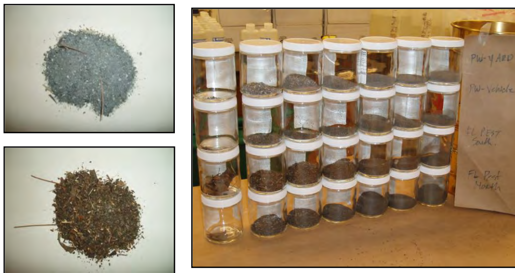
Photographs on left show the samples before sieve analysis was conducted; top is contents from the inlet filter at PW Yard and bottom is the contents from the FP South inlet filter. The photograph on right displays the contents retained by each sieve size for each stormwater inlet filter.
