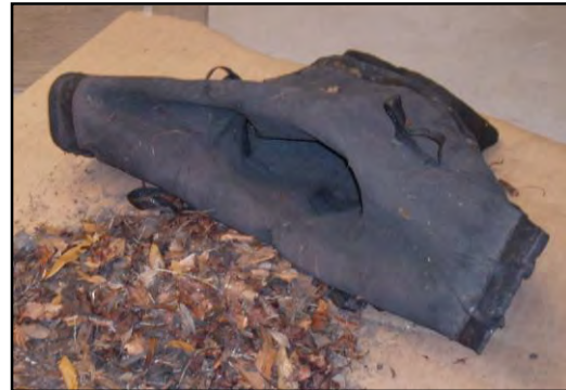
Ultra-DrainGuard Oil and Sediment filter and contents after removal from one of the stormwater inlets
