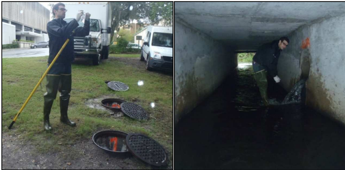
Figure A-4. Sample collection from the baffle box chambers, SWB1, (left) and the outfall pipe, SWB1OUT, under the pedestrian bridge in Sweetwater Branch Park (right). August 27, 2012
