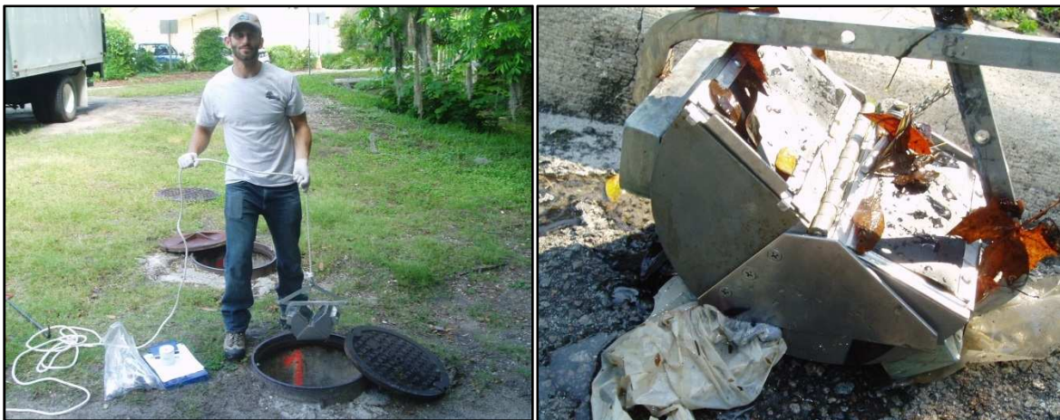
Figure A-5. Sediment sample collection from the baffle box chambers, SWB1 (left) and the Petite Ponar sampler with sample collected from the CDS unit at SWB8 (right). June 4, 2013 and August 5, 2013
